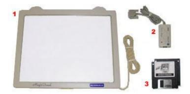
A basic touch screen has three main components: a touch sensor, a controller, and a software driver. The touch screen is an input device, so it needs to be combined with a display and a PC or other device to make a complete touch input system.
