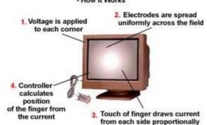
A capacitive touch screen consists of a glass panel with a capacitive (charge storing) material coating its surface. Circuits located at corners of the screen measure the capacitance of a person touching the overlay. Frequency changes are measured to determine
